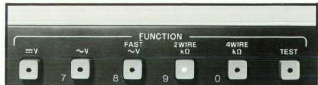
Fig. 3. Programming codes for systems control are labeled on the front panel. An underlined letter, such as the F shown here, is the program code for a group of pushbuttons. A particular pushbutton is specified by its position in the row counting from the left (e.g. the number 3 for FAST ac volts).
