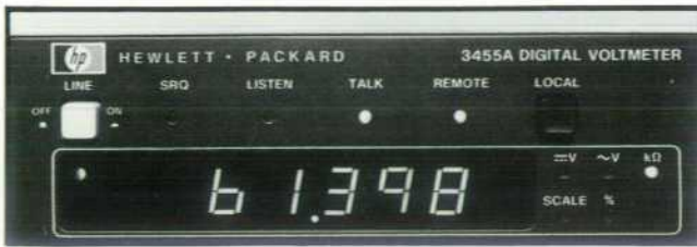
Fig. 4. Indicator lights show the status of the instrument when operating on the HP interface bus.
