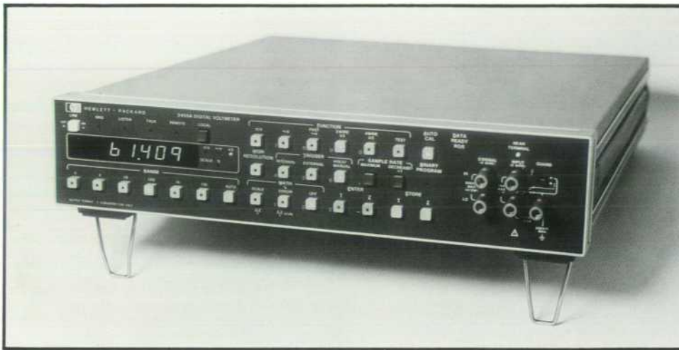
Fig. 1. Model 3455A Digital Voltmeter measures dc volts, ac volts, and ohms under either manual or systems control. Indicator lights in the pushbuttons show the ranges and functions selected manually or remotely through the HP Interface bus.
